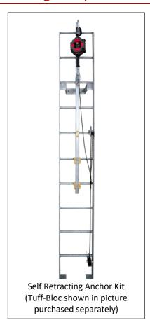
Self-retracting lanyard anchor kit, designed to be installed on the rungs of a ladder. Systems shall be designed to limit free fall, swing fall and maximise fall clearance. Where possible, systems should be installed as close to the centre of the ladder or climbing zone as possible. Use in conjunction with SafetyLink's Tuff-Bloc's.
