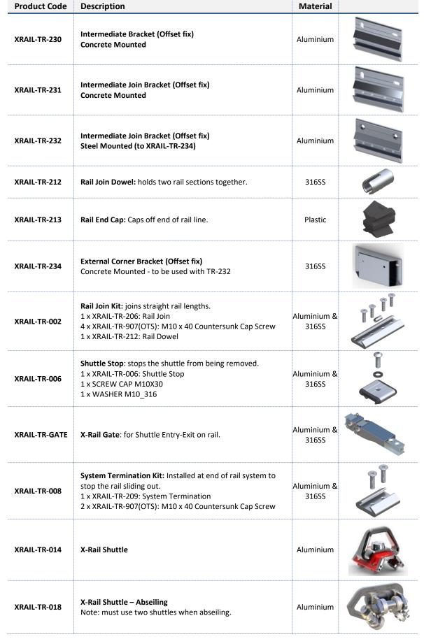
CONCRETE & STEEL – OFFSET FIX X-RAIL – COMPONENTS & KITS
