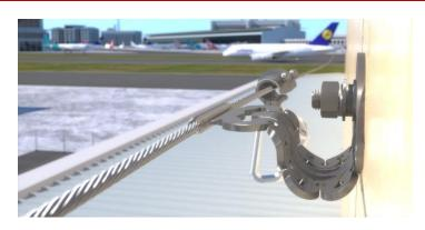
The FrogLine Wall Mounted System is a wall mounted horizontal lifeline installed into concrete construction. The system is equipped with SafetyLink's engineered energy absorbing intermediate and end anchors to minimise loads on both the user and structure in the event of a fall. The continuous connection via the Overhead Shuttle System on the 8mm stainless steel cable provides protection for up to four (4) users per system, two (2) users per span.
