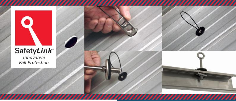
The Retro*Link* is an abseiling anchor point designed for use on metal roofing/steel purlin structure. Installation is a simple task requiring no access from underside of the roof.
