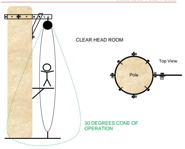
PoleLink Anchor must only be installed whilst in a Safe Work Position by a suitably competent person from an elevated work platform (EWP) or by appropriate rope access (RA) methods only. All tools should be secured with leash/lanyards to prevent accidental dropping from heights. A safe work exclusion zone needs to be created at the base of the installation site.
