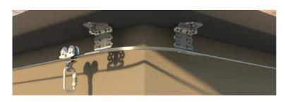
The FrogLine Overhead Mounted System is an overhead mounted horizontal lifeline installed into concrete construction. The system is equipped with SafetyLink's engineered energy absorbing intermediate and end anchors to minimise loads on both the user and structure in the event of a fall. The continuous connection via the Overhead Shuttle System on the 8mm stainless steel cable provides protection for up to four (4) users per system, two (2) users per span.
