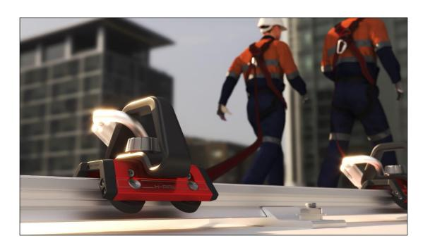
The SafetyLink X-Rail is a Rigid Anchor Line suitable for use as part of personal fall protection system. The X-Rail offers a Horizontal Rigid Anchor Line with one or multiple Mobile Anchor Points for attaching to. The X-Rail can be installed in three orientations; Overhead, Wall and Floor mounted and can be used for Fall Arrest and Abseiling purposes.
